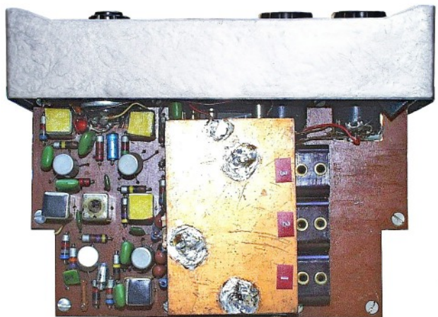
Internal view of VR 17 showing receiver board (left) and three crystal sockets for the transmitter (right).
