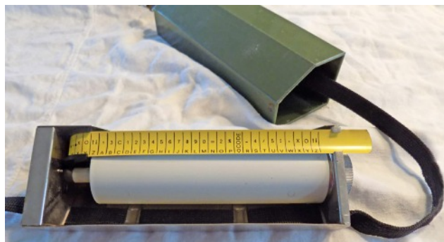
Internal view of the M-75 cipher unit showing the printed tape measure and drum.
