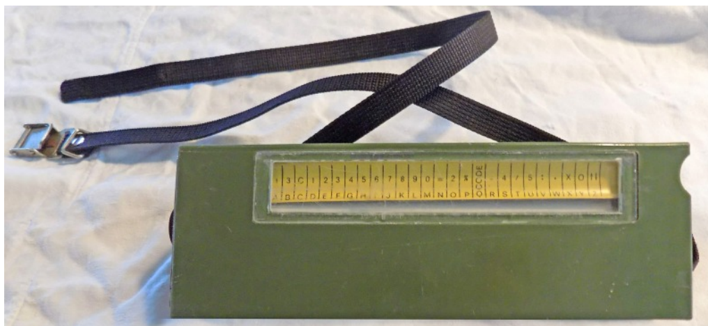
Issued with VR 17 stations was a remarkable manually operated cipher unit M-75. It was comprised of a retractable tape measure printed with the alphabet, numbers and symbols, and a rotating drum. Not a high security and unbreakable cipher system, but for simple field use under any weather condition, without mechanical or electrical complexity, suitably only for immediate and short term use.
